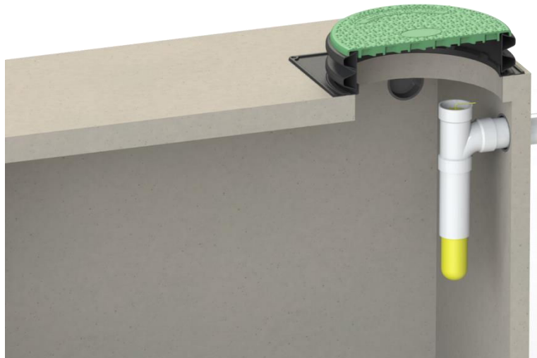
Figure 45, Filter Installation into Tee Baffle
