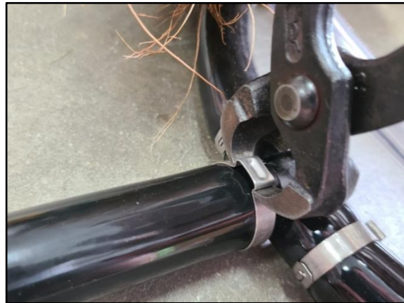
Figure 12, Connecting Ballast Sections of Bio-Brush Clusters
