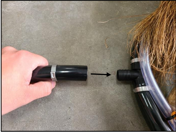
Figure 12, Connecting Ballast Sections of Bio-Brush Clusters
