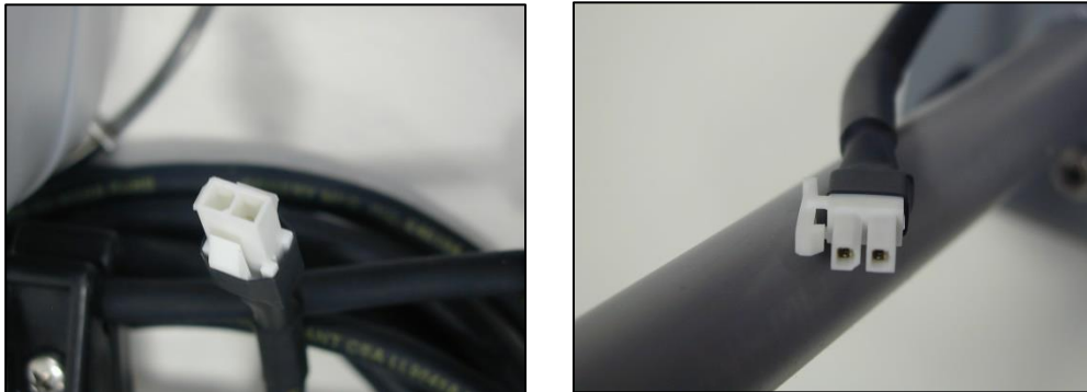
Figure 36, Float Switch Connector (Left) and Aero-Alert Connector (Right)
