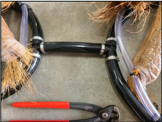
Figure 12, Connecting Ballast Sections of Bio-Brush Clusters
