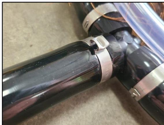
Figure 13, Bio-Brush Ballast Connections and Crimping Process
