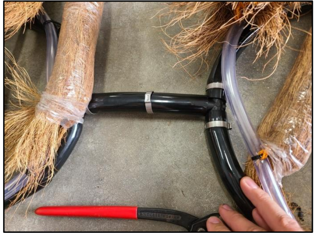
Figure 12, Connecting Ballast Sections of Bio-Brush Clusters
